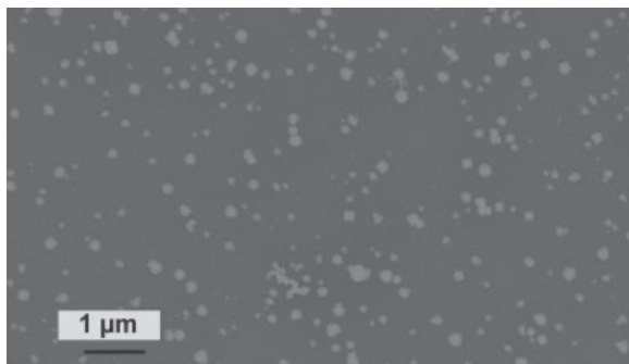
Figure 2.101 Photoelectrodeposition of Pt for preparation of a nanoemitter photocathode: (a) SEM image of porous oxide matrix on Si(100); (b) deposition protocol: solution, 1 mM \text{PtCl}_6^{2-} , 0.1M \text{K}_2\text{SO}_4 , pH 3.8; light intensity, 130\text{ mW cm}^{-2} , W-I lamp; (c) SEM image after Pt deposition.
